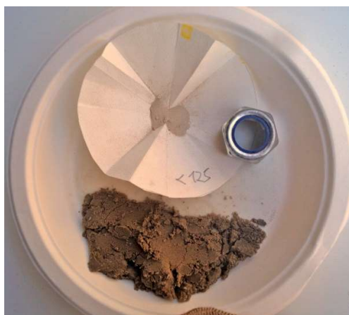
Figure 9. Sandy clay from the Argille di Fangario formation (see text) - Sandy fraction, 125\mu - 64\mu interval, visual proportion of sinking and non-sinking (on filter paper) residue.
